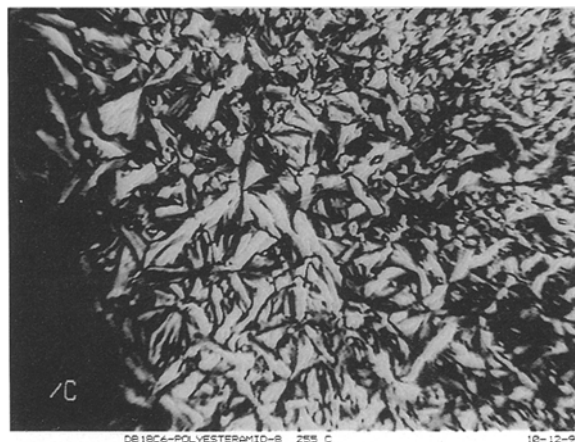
Figure 1: Optical micrograph of polyesteramide Id , 255 °C, 160 X
